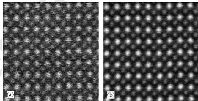
Fig. 7. High-Angle annular dark field lattice images of  $\text{SrTiO}_3$  recorded on our monochromated Techni-T 200 kV with a 40 mrad collection angle, and 9.6 mrad incident angle. The bright atoms are Sr, and the fainter ones are Ti. (a) at  $32\ \mu\text{s}/\text{pixel}$ , (b) The average of 10 cross-correlated images, each recorded at  $32\ \mu\text{s}/\text{pixel}$ . Both images are  $33\ \text{\AA}$  full scale.
