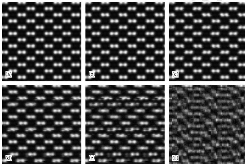
Fig. 3. Simulation of the effect of AC noise on the  $x$ -scan for Annular dark field STEM images of [1 1 0] Silicon using the field sensitivities determined from Fig. 2. (a) no noise, (b) 0.2 Å p-p (0.15 mG r.m.s.), (c) 0.4 Å p-p (0.3 mG r.m.s.), (d) 1 Å p-p (0.7 mG r.m.s.), (e) 2 Å p-p (1.4 mG r.m.s.), (f) 2 Å p-p in both the  $x$  and  $y$  scan directions. The imaging conditions are assumed to be 200 kV,  $C_s = 0.5$  mm, 10.5 mrad objective and 50 mrad ADF inner angle at optimal defocus.
