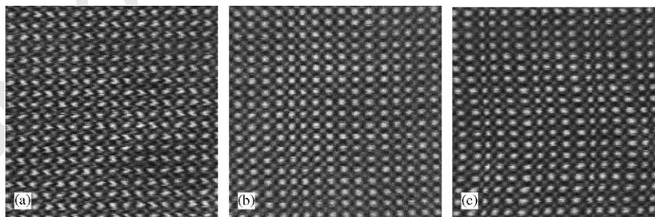
38 Fig. 1. The effect of a modest AC field on an ADF-STEM image of SrTiO<sub>3</sub> recorded on a JEOL 2010F. (a) The image is recorded without any
